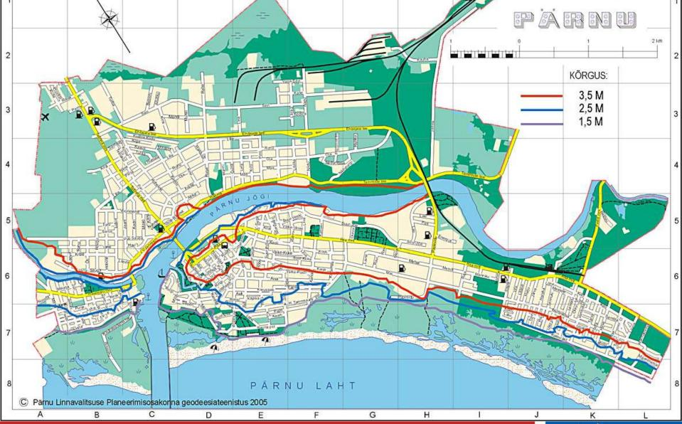
The blue line marks flood up to 2,5m, the red line marks rise of sea level up to 3 metres.
